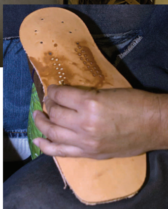
One of the skilled craftsmen at Anderson Bean Boot Company using lemon wood pegs to secure the steel shank in place on a pair of \frac{3}{4} welted Anderson Bean Boots.
